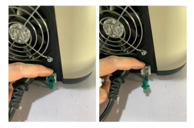
Connect the other end joint of the transfill tube into the port of transfill until you hear it click and secure into place.
