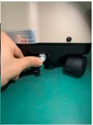
Press the metal shrapnel on the port of the transfill. The plastic plug will loosen and pop out.
